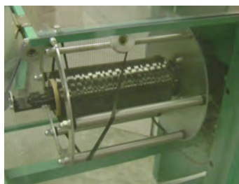
Picture shows special cage system to twist carbon fiber
