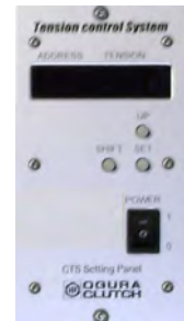
Picture above shows basic tension setting interface for all PC series creels.
