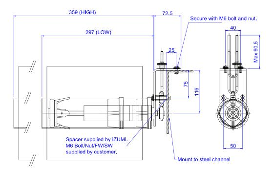
Model ST-5N, 2N, 1N have identical mounting dimensions.
